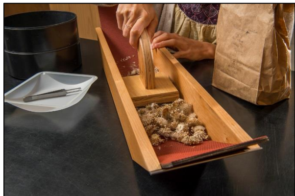
Figure 5. Using the seed boat to clean Asteraceae seeds. This method is useful to remove the pappus on seeds. Sieves can be seen on the left.
