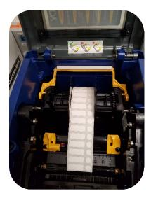
Pull the labels over the shiny black roller and close the 2 yellow alignment guides so the arrows are aligned with he edges of the label sheet.
