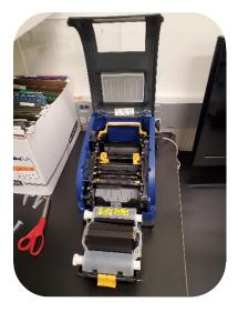
Place the roll of labels into the printer. The roll is designed to only fit into the printer the correct way. Pull the labels over the shiny black roller and wind the reel to retract any excess slack. Labels can be found above the PCR Workstation in the box labeled 1.5 mL eppie tubes.
