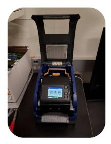
Press the yellow center latch toward the front of the machine and pull forward to fully open the printer.
