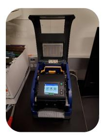
Press the yellow center latch toward the front of the machine and pull forward to fully open the printer.
