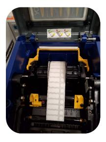
Pull the labels over the shiny black roller and close the 2 yellow alignment guides so the arrows are aligned with he edges of the label sheet.
